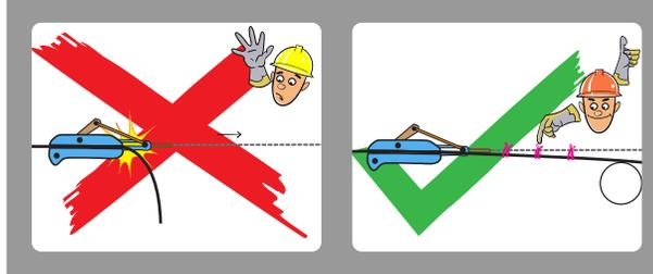
Don't allow the conductor tail or the deadend to fall or droop unsupported while handling the conductor. If the tail is not controlled, it will damage the core at the back of the grip. Don't use pocketbook grips or short-jaw parallel jaw grips.
